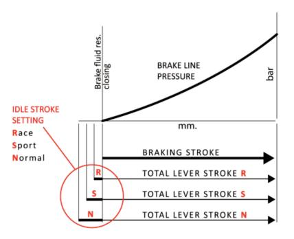
The effective (efficient) lever stroke is the total lever travel - to produce a certain pressure in the brake circuit- minus the idle stroke that is the distance between the main seal of the piston in neutral position and the inlet hole of the brake fluid (coming from the reservoir).
